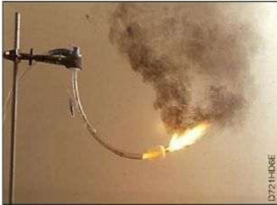
Figure 2. Demonstration of rocket-like flames shooting from a tracheal tube caused by laser ignition of the tube with 100% oxygen flowing. Image provided courtesy of ECRI Institute.
